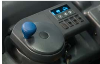
Electronic steer-by-wire system with small diameter steer tiller arm provides quiet, responsive maneuvering
