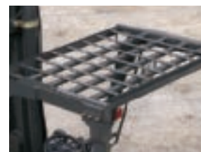
Head guard with front/rear gutters
