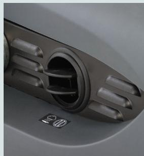
Wet sweep bypass protects the filter from water fouling when sweeping in wet conditions.
