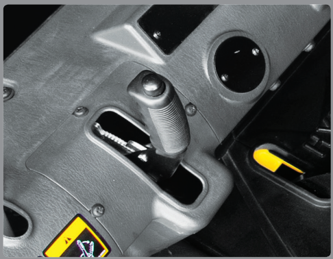
Parking brake Ratchet type parking brake requires less effort the operator to set.
