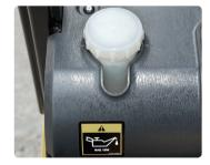
Brake Fluid Reservoir With Level Switch
