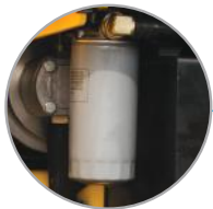
Hydraulic Return Oil Filter is Easily Accessible
