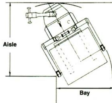
Note: Aisle dimensions listed above assume the bay width to be straddle OD plus 2" (1" on each either side of straddle leg). Straddle OD is the load width plus 10"
